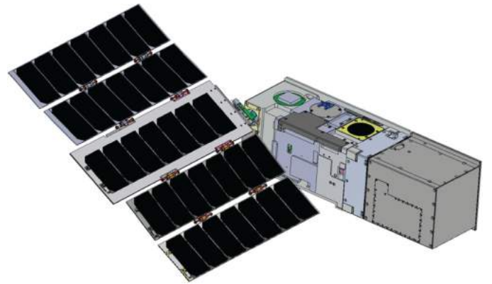
Figure 22: TROPICS space vehicle showing CubeSat bus, radiometer payload, and deployed articulated solar array
